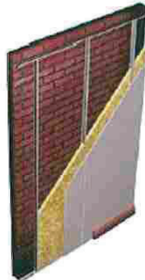
Figure 2 Typical Independent Wall Lining System
